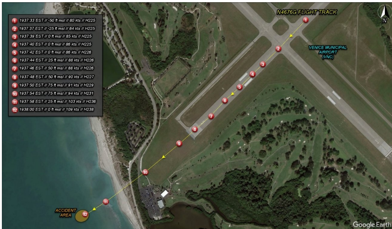
Figure 1. Preliminary ADS-B flight track information
