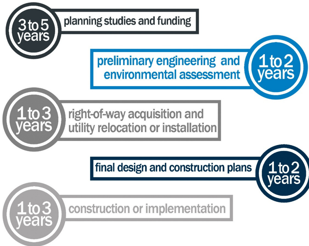
Figure 6-1. Typical Project Development Process and Timelines
