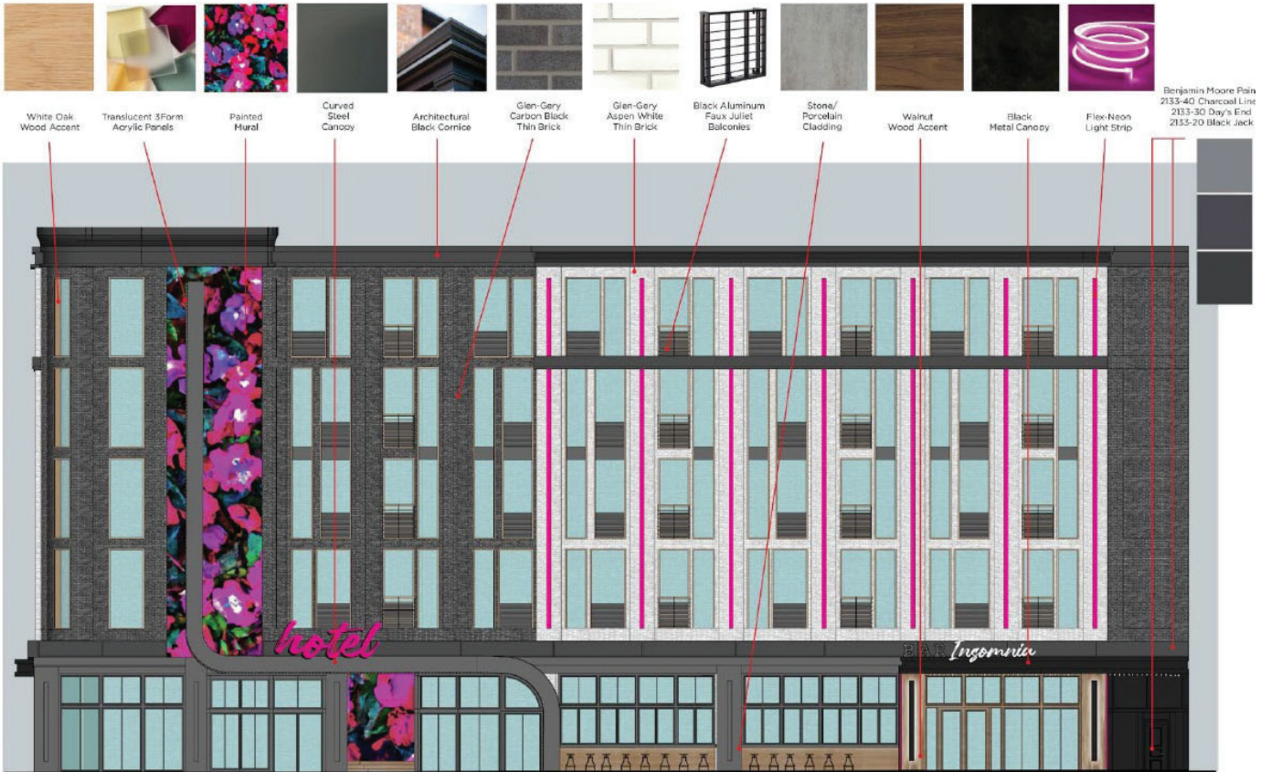
Façade materials of proposed building. (Applicant)
