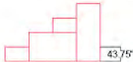
There are three primary alternatives for a more accessible access point. The first alternative is a ramp with a 5% grade. This is the maximum grade allowed for a ramp before American with Disabilities Act (ADA) standards must be applied (4.8 Ramps, ADA). It consists of four switchbacks, each 72'-11" by 6'-0" with three landings, each 5'-0" by 12'-0" These dimensions accommodate two wheelchairs side by side.
