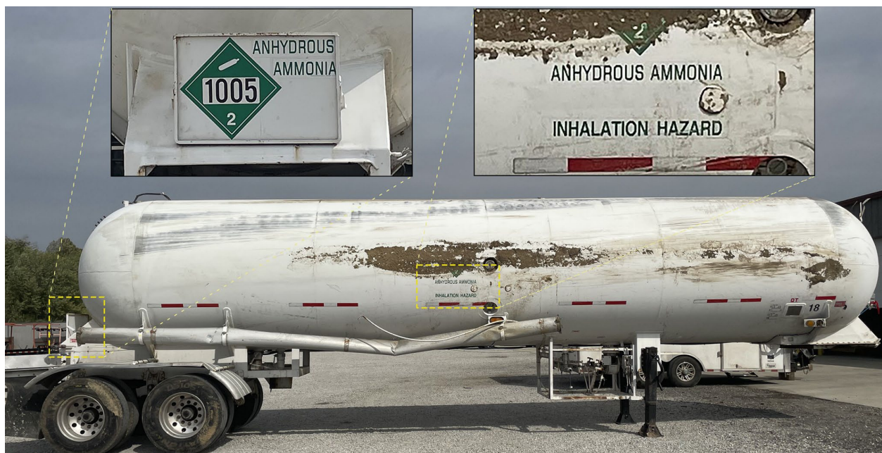
Figure 8. Marking and placarding on the cargo tank. The left side of the cargo tank does not have soil deposits and the marking and placarding is clearly visible.
