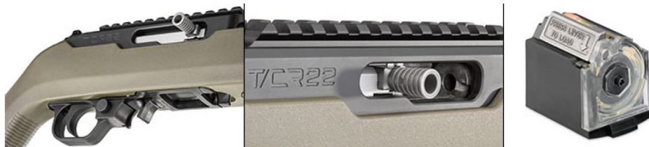
(l.) A quick glance at the T/CR22 shows its similarities to the Ruger 10/22.. (ctr.) Generously sized and easy to operate, the bolt handle also locks back easily. (r.) Familiar in appearance, the T/CR22 magazine was rather difficult to load.
