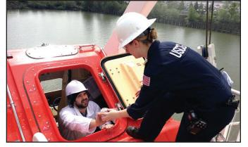
Photo courtesy of Petty Officer 3rd Class Valerie Walker Lt. Katherine Brodie, Marine Inspector at Coast Guard Marine Safety Unit Portland, inspects an emergency fishing tackle box kept in the lifeboat aboard the vessel Port Belmonte, during a Port State Control exam at the Port of Portland, Ore., April 30, 2017. Brodie inspects whether the lifeboat contains fresh and complete provisions to sustain all crew members in the event of an order to abandon ship.
