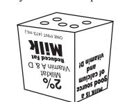
Punch five small holes in the bottom of the carton for drainage.
