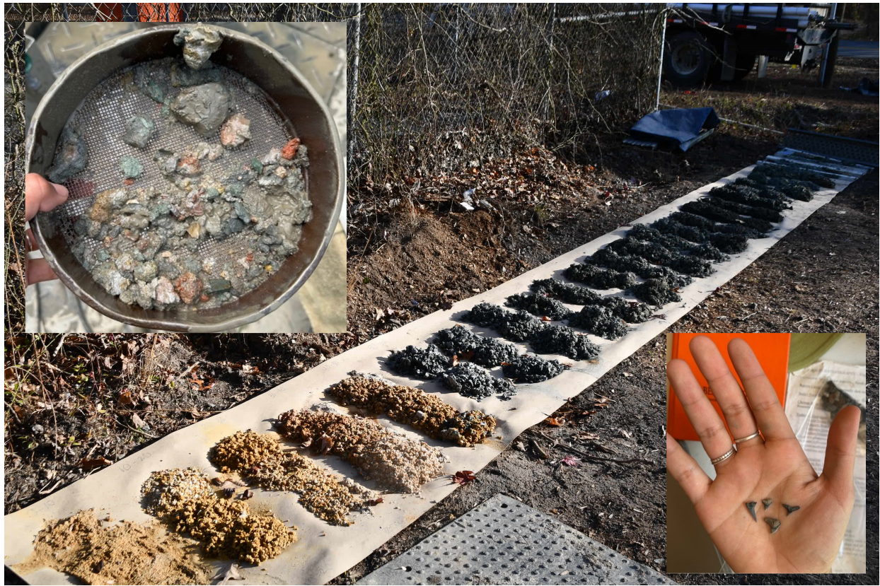
(c) Drill cuttings samples reconstructed into groups representing 10-foot intervals of depth below land surface, for detailed description and logging. Inset images show the sampling sieve (left) and fossil shark teeth (right). Formations and aquifers are determined using these samples, borehole geophysical logs, and other data.
