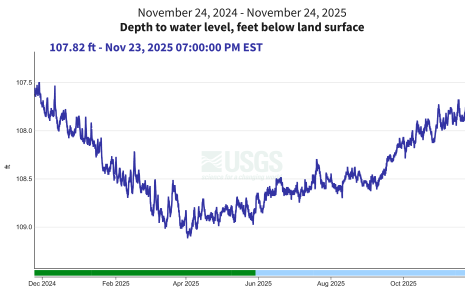
Figure 22: Hydrograph for SOW 252A in Isle of Wight County, showing water levels in the confined Potomac aquifer and variation caused by pumping effects (USGS, 2024).
