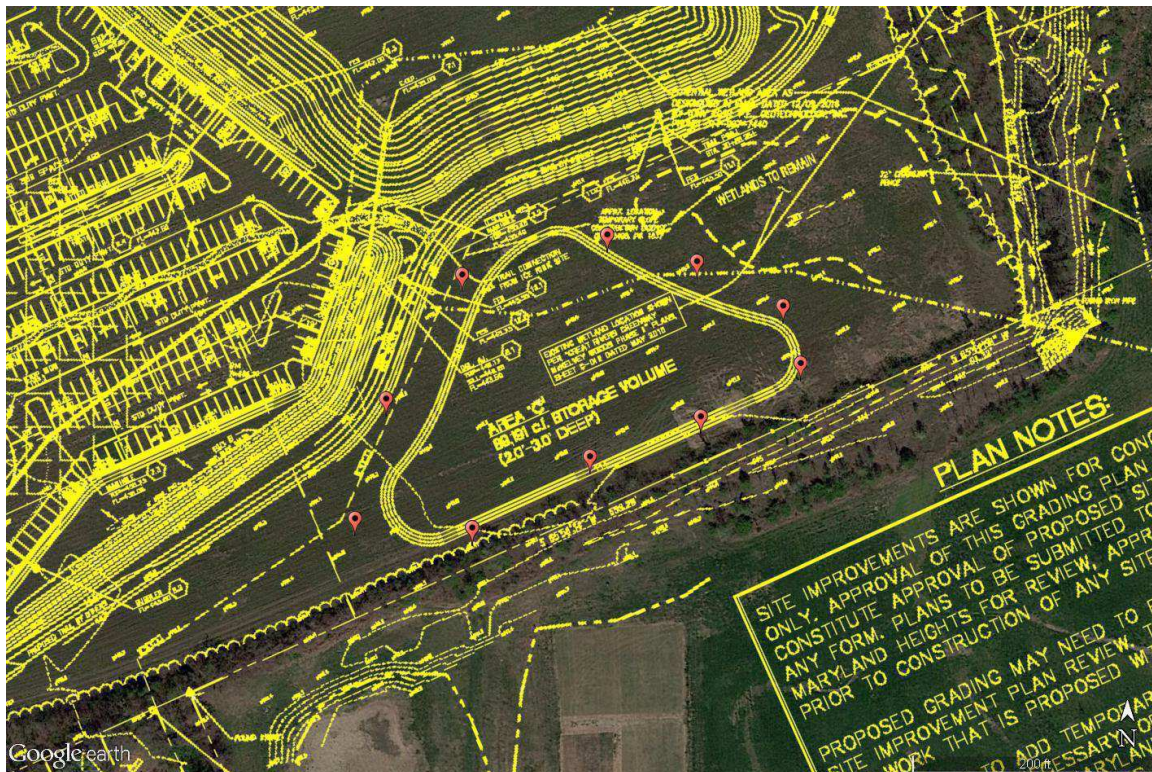
Figure 9. GPS coordinates collected around the perimeter berm of Area C in Google Earth (top; imagery dated 4/2/2016, prior to the start of grading activities on the site) and superimposed on the grading plan for the ice center (bottom).
