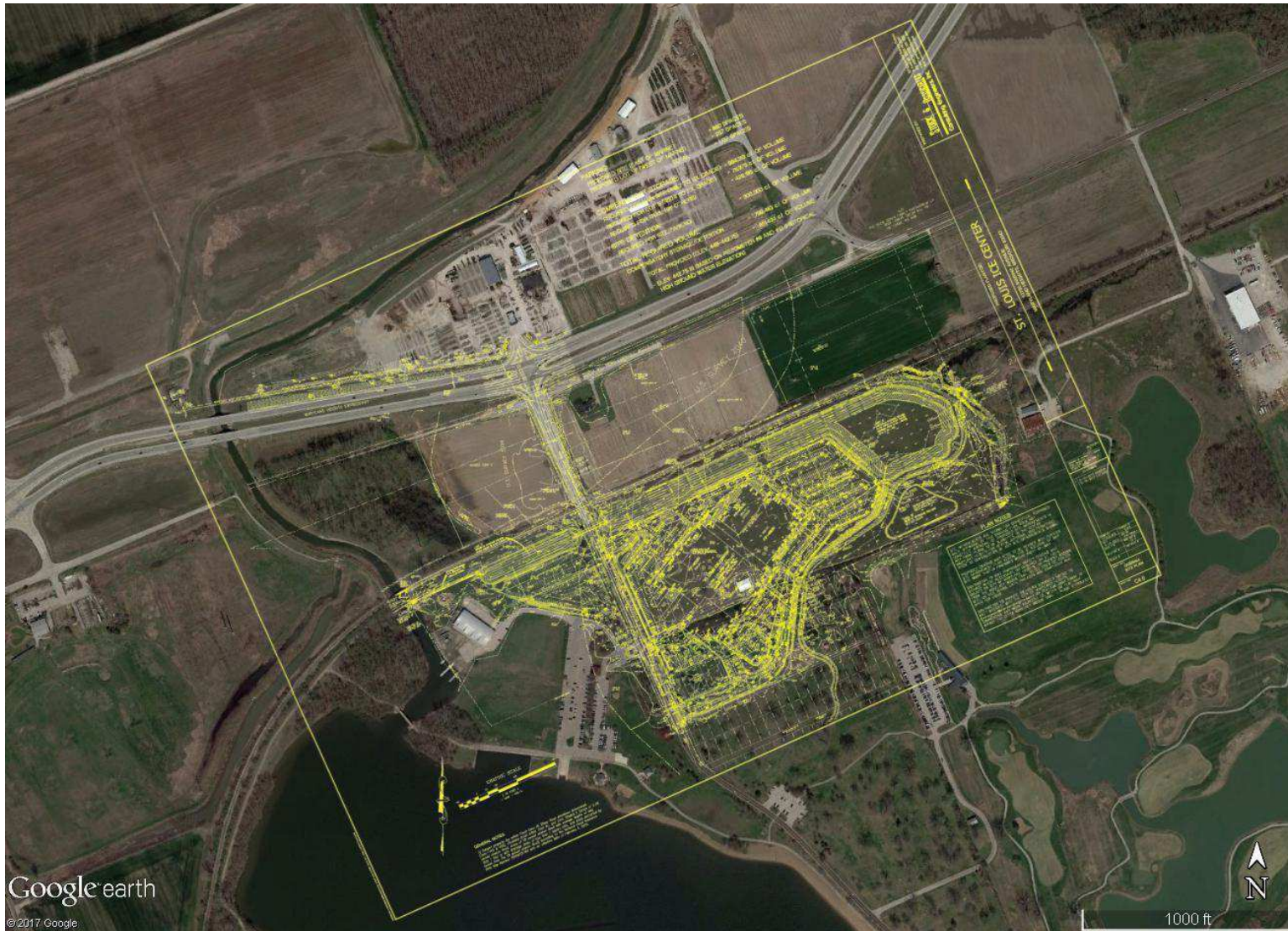
Figure 2. Ice center grading plan as a georectified image overlay in Google Earth (line color changed for enhanced visibility).
