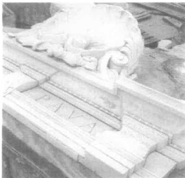
Figure 23. Production molds (left) made of durable rubbers backed with wood and plaster supports are used to fabricate new cast stone. Production molds may be made from original elements which have been repaired with epoxies and plaster, or from new plaster mockups, (below).
