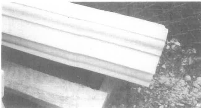
Figure 24 Separation of an interior rubber mold from a plaster mother mold during casting may result in rippling or irregularity of the completed casting.
