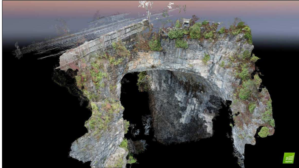
Figure 9. A still image taken from a point cloud animation of the upstream-side of Natural Bridge. Point clouds like this are georeferenced allowing for quantitative measurements to be made, including discontinuity orientations for stability analyses.
