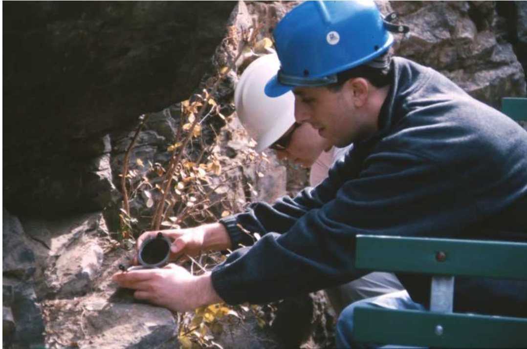
Figure 15. Manual collection of discontinuity orientation data by Radford University graduate students at Natural Bridge in 2000.
