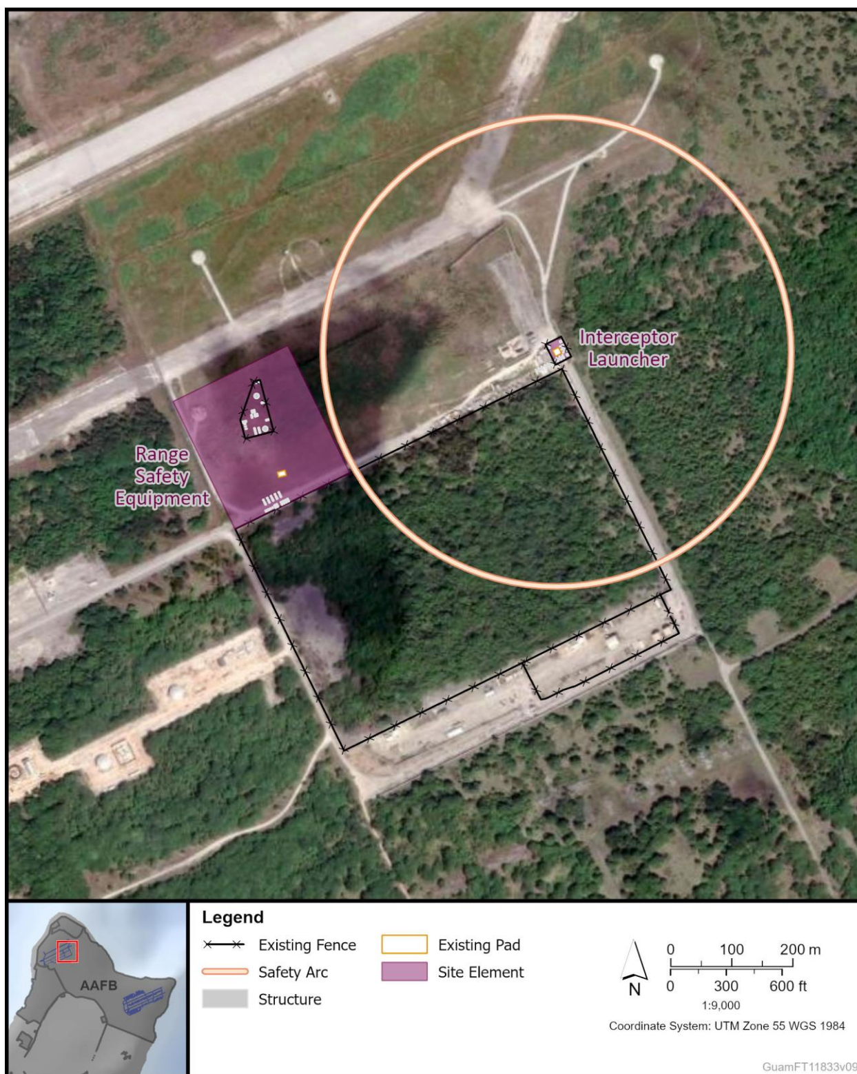
Figure 2.1-4: FEM-02 Explosive Safety Quantity Distance
