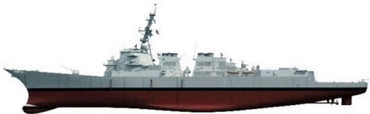
Arleigh Burke Flight IIA DDG 79 505' (153.9 m) 8,627 tons Beam 59' (18 m)
