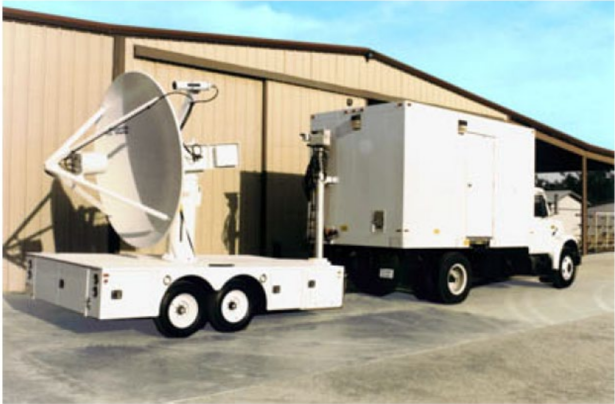
Figure D-2: Single Transportable Telemetry System Unit
