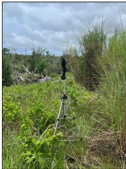
Figure 2-1: Typical SLM Setup
