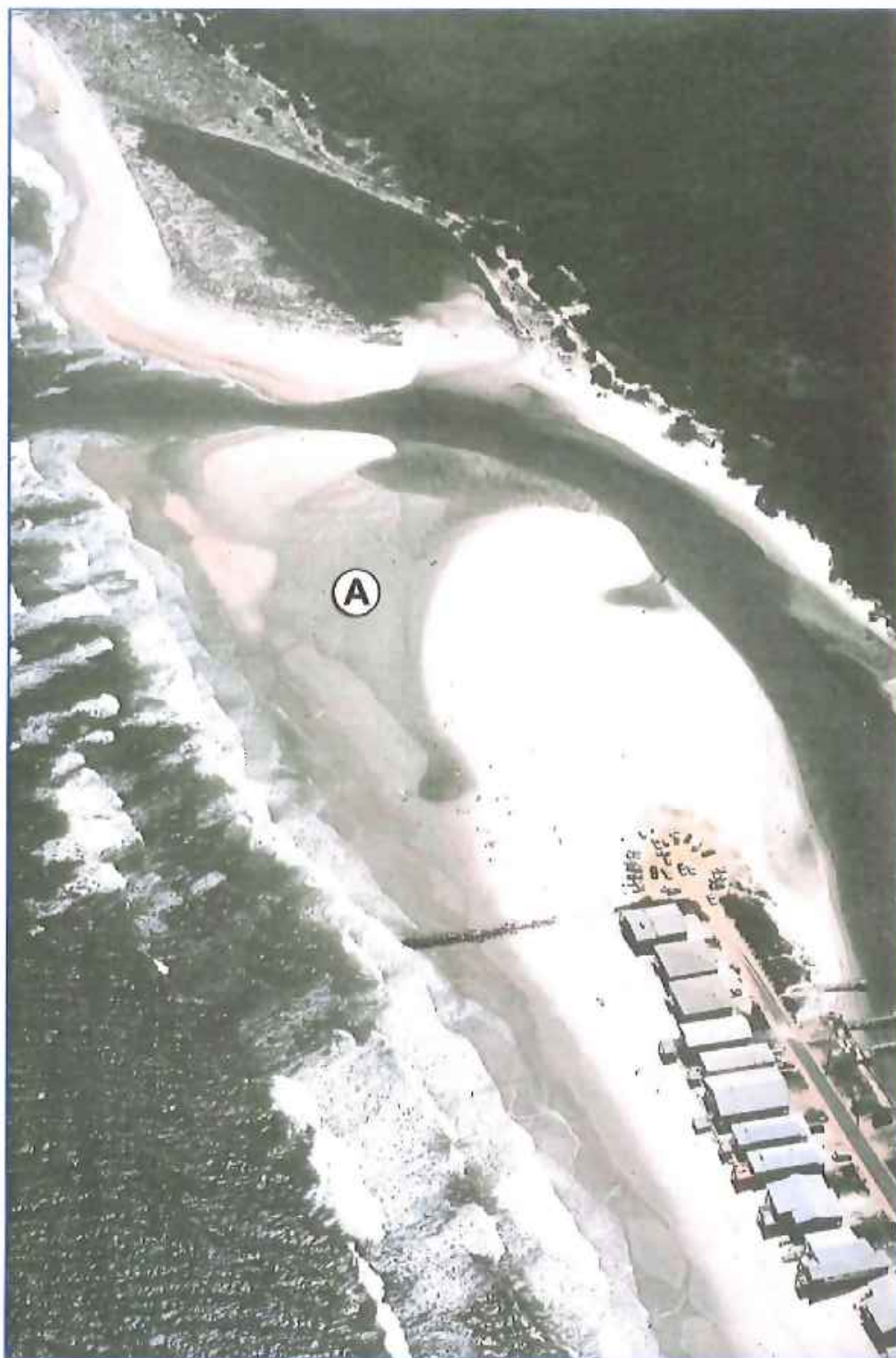
FIGURE 13. Pawleys Inlet at low tide on 15 May 1985 when the channel was positioned about 1,200 ft south of Groin #1 (visible near the lower center of the photo). Note the intertidal shoal platform (area A) on the updrift side of the inlet which acts as a fillet and helps maintain the spit. An abandoned channel ("cat-eye" pond) is at the top of the image.
