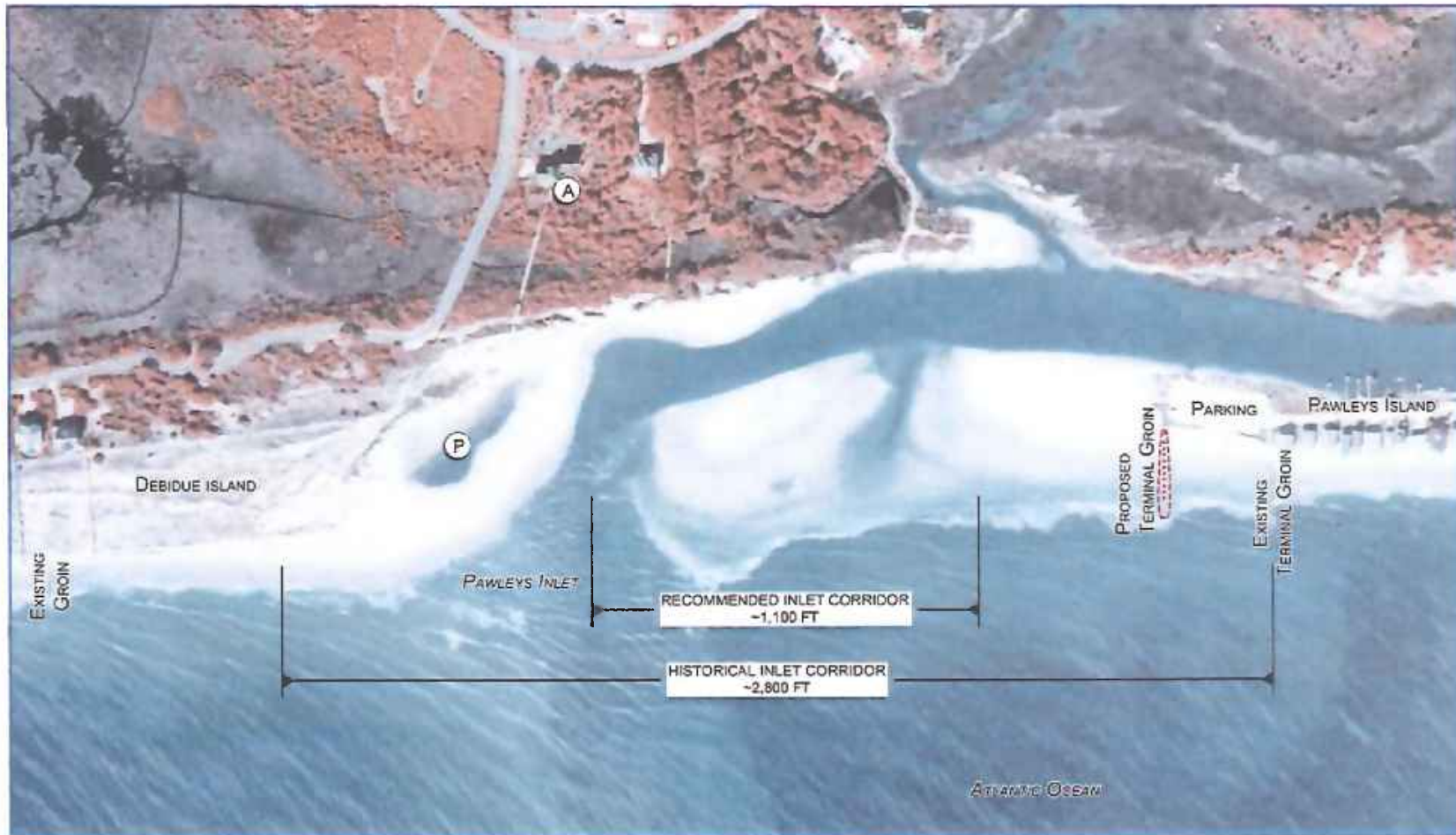
FIGURE 1. Pawleys Inlet in March 2006 showing the area from Groin #1 (labeled Existing Terminal Groin) to an existing groin at the northern end of Debidue Island. For the past 60 years, with one exception, the inlet has remained within the indicated historical corridor. Hurricane Hugo (September 1989) breached Pawleys spit 2,200 ft north of the terminal groin and shifted the inlet until it was closed in October 1989. CSE (letter from TW Kana to H Faison dated 4 September 2009) recommended a narrower inlet corridor be designated for purposes of avoiding encroachment on existing development. Area "P" is an abandoned former channel. An incipient channel through the spit is evident in the area above the word "corridor." (Photo courtesy of SCDNR)
