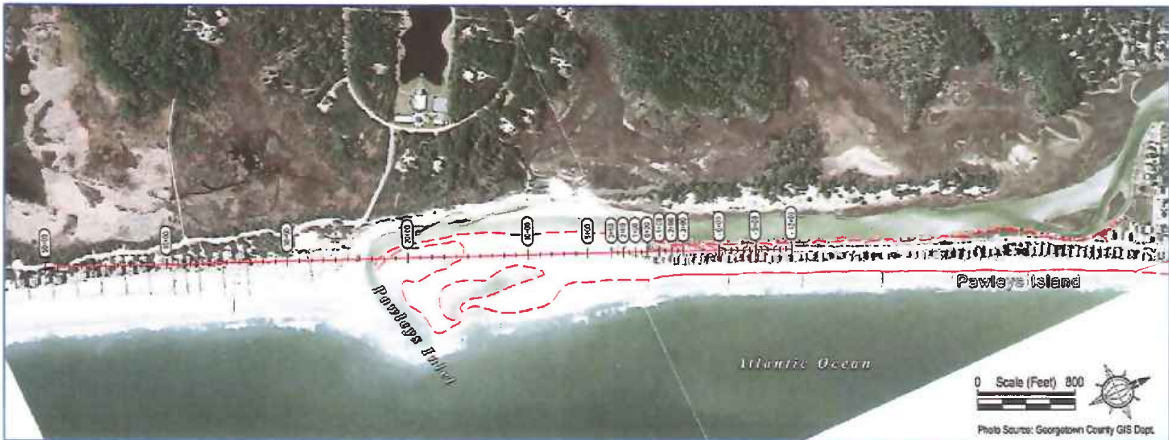
FIGURE 5. Most recent vertical aerial photograph showing position of Pawleys Inlet in March 2009 (courtesy of Georgetown County GIS Department). Note proximity to Beach Bridge Road, an access road within the Prince George community on the south side of the inlet. The PGCA installed emergency shore protection (buried) in August 2009 landward of jurisdictional setback lines to protect the road and utilities.
