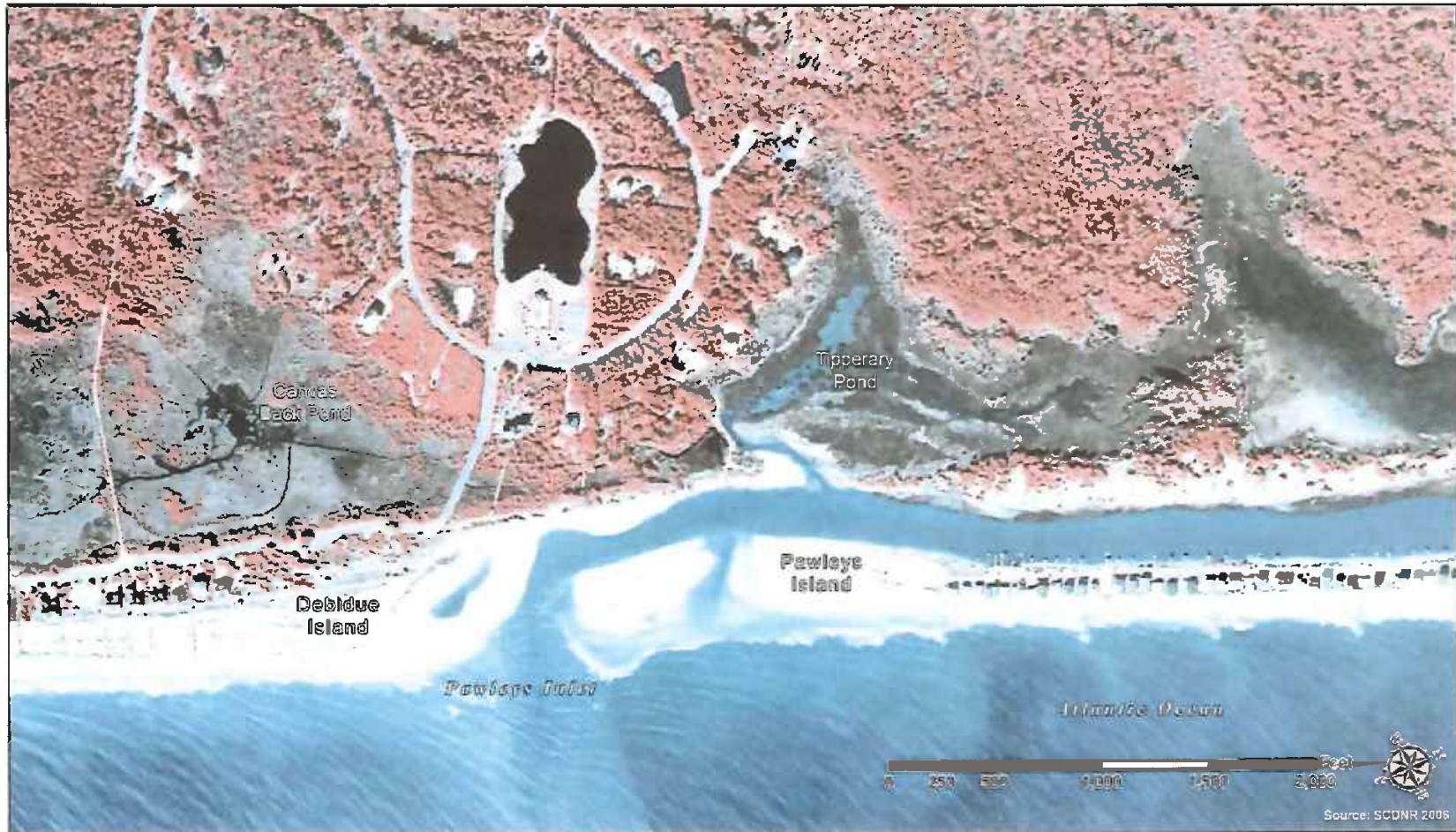
FIGURE 15. Pawleys Inlet in March 2006 showing (right to left) an incipient channel through the end of Pawleys spit at ~1,000 ft south of Groin #1, the main entrance channel ~2,000 ft south of Groin #1, and a remnant channel ("cat-eye" pond) on the Debidue Island side of the inlet. Note the breach of the mainland shoreline north of Pawleys spit (dry-sand area). The breach channel has created a connection with the large brackish water impoundment, Tipperary Pond. Continued southerly migration of Pawleys Inlet increases the likelihood of a breach into Canvasback Pond, which contains extensive fresh-water wetlands.
