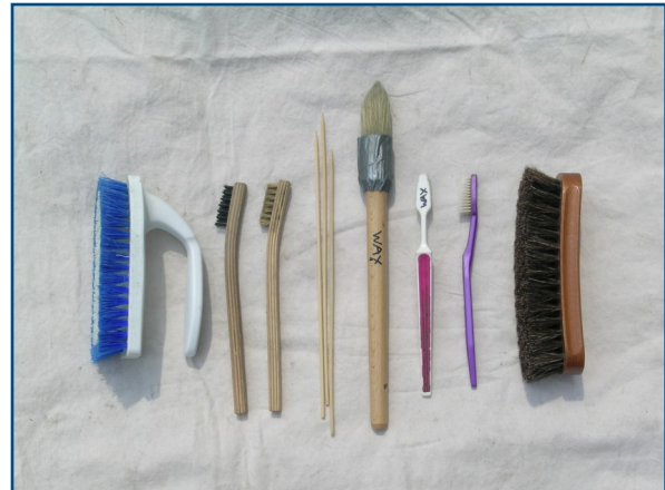
Materials used for cleaning and waxing: scrub brushes, bamboo skewers, waxing brush, toothbrushes for buffing, and horsehair shoe polishing brush. (Judith M. Jacob, NPS)
