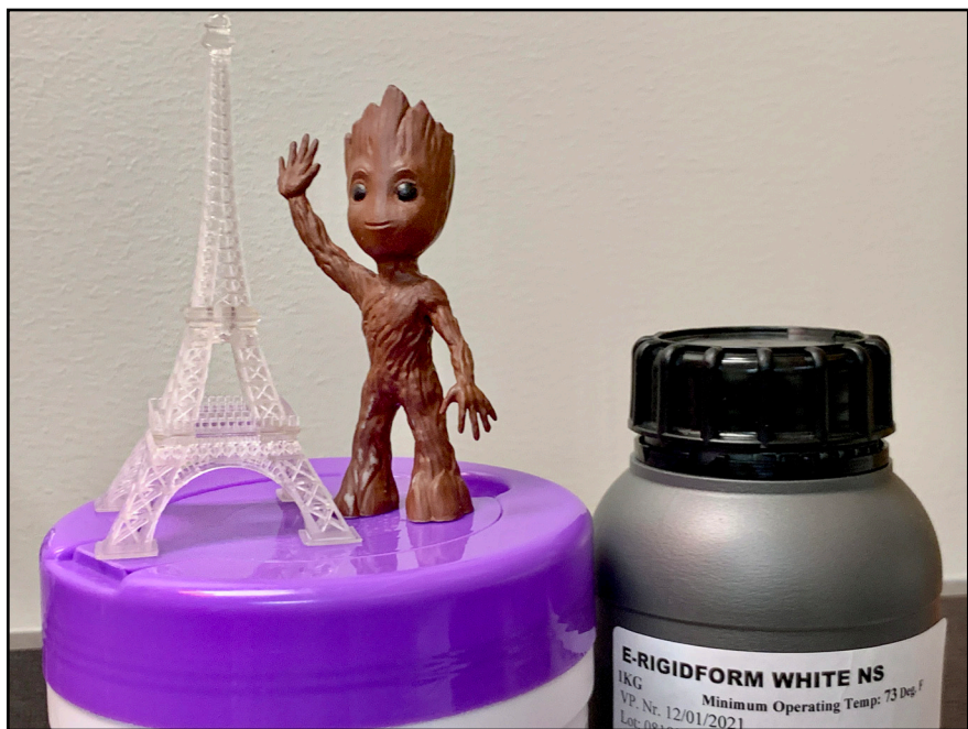
These sample resin figures just inches high, called "rapid prototypes," were created by Arius's students on the computer and produced with a small EnvisionOne 3D printer, most often used in dentistry. This widespread manufacturing process has increasingly important uses in areas from aerospace to fine art to medicine.
