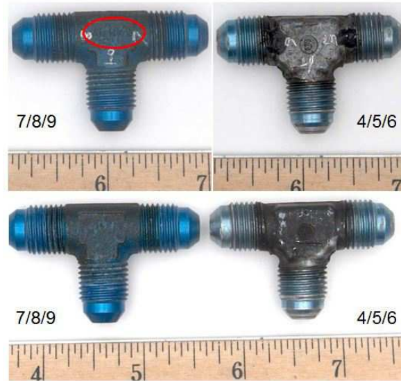
Figure 10. T-Shaped Fittings. Red circle indicates a correct marking (Tab J-34).
