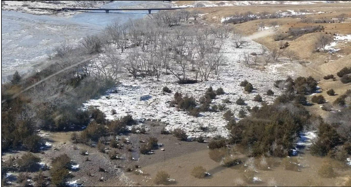
Figure 4.15 – Ice deposit on north side of river downstream from the highway (NPPD photo).
