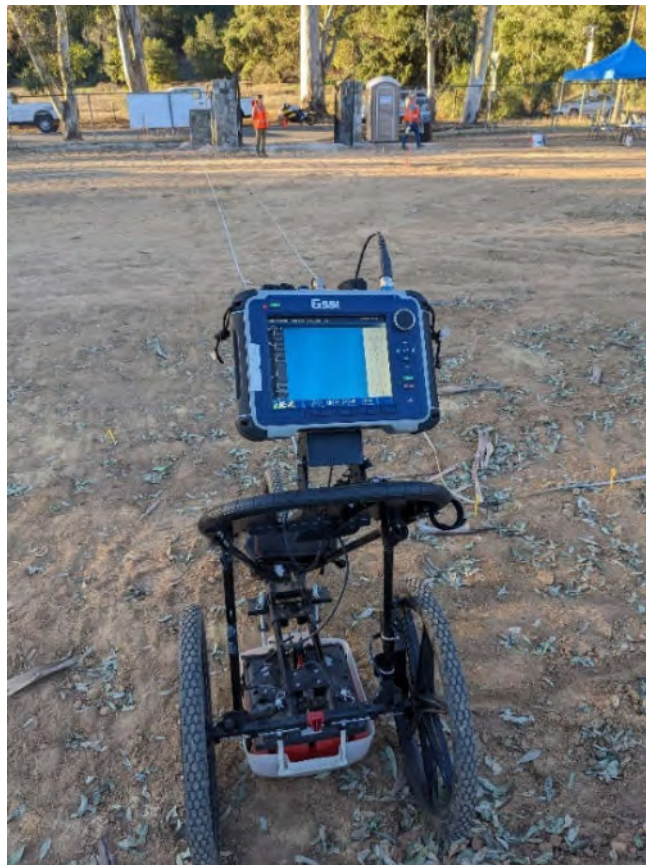
Figure 1. Start corner (0/0) in Grid 6, facing south towards gate. SIR4000 GPR system in foreground.
