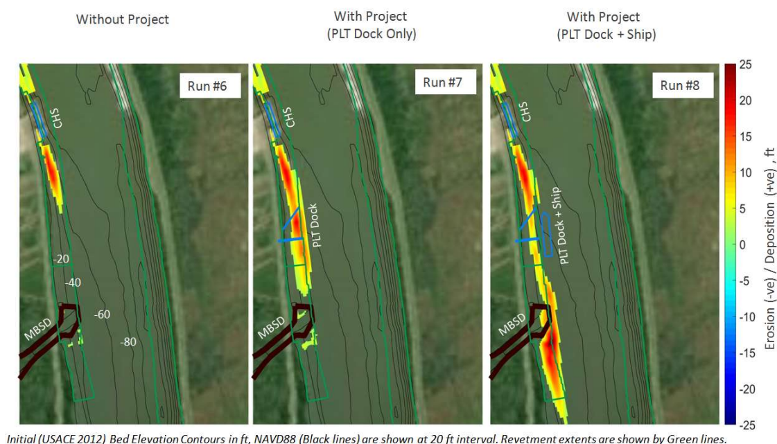
Figure 5.26. With-morphology-change, non-erodible initial bed diversion open (Runs 6, 7 and 8): deposition extents and depths at the end of 1 year of diversion operations, after immediate opening of the diversion under Without-Project, With-Project (PLT Dock only) and With-Project (PLT Dock+Ship) scenarios.
