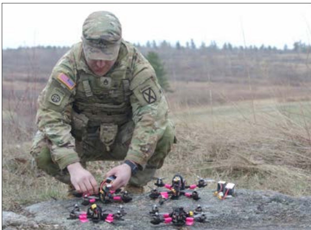
Above: Staff Sgt. Christopher Heath, a tactical unmanned aircraft systems specialist for Foxtrot Company, 10th Combat Aviation Brigade, conducts a preflight check for UAS on Monday at Fort Drum. U.S. Army photo by Spc. Isaiah Mount
