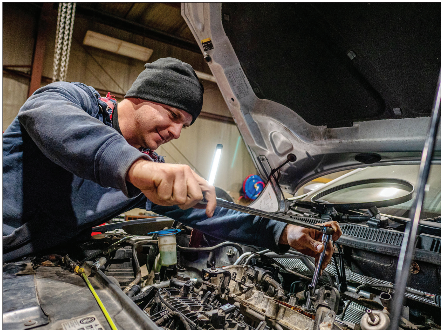
Justin Ernst, owner of C&J's Repair Shop and SEATS Transportation, fixes the engine of a Volkswagen Jetta that was damaged after the owner ran it without oil. ZACHARY CANAPERI/NNY BUSINESS
