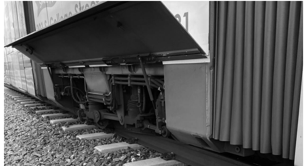
Derailed LYNX light rail | Courtesy of Charlotte Area Transit System
