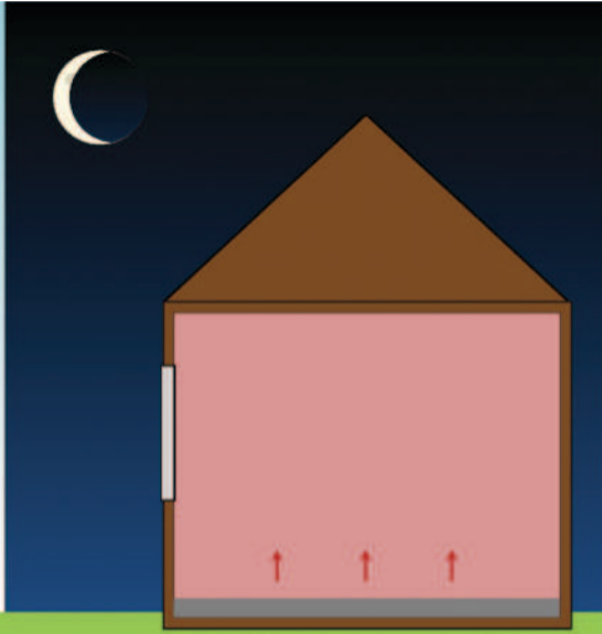
Night: Thermal mass in floor releases heat into room
