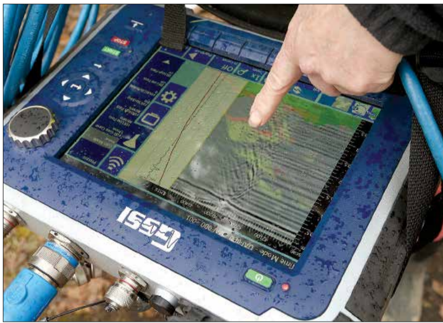
Stephanie Saari, with the Army Corps of Engineers Cold Regions Research and Engineering Laboratory, explains the readings on the ground-penetrating radar she was calibrating as UAF film students and researchers with CRREL scan for buried fossils Wednesday morning on UAF property off of Farmers Loop Road near Ballaine Lake. ERIC ENGMAN/NEWS-MINER PHOTOS
