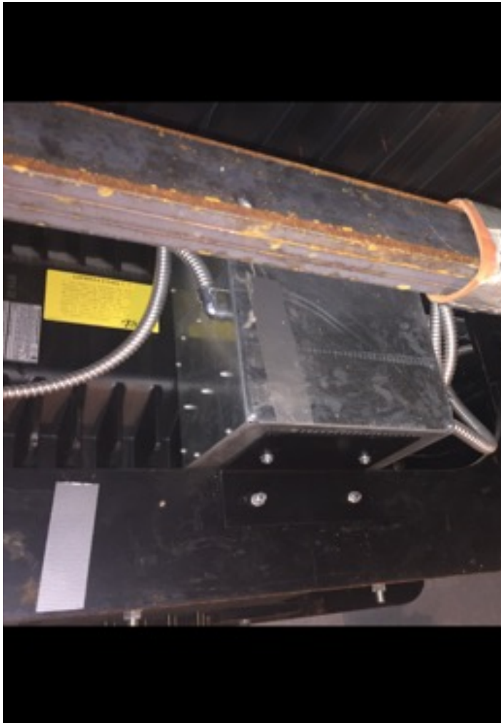
Typical Rust on Equipment in Overhead on Express Cars
