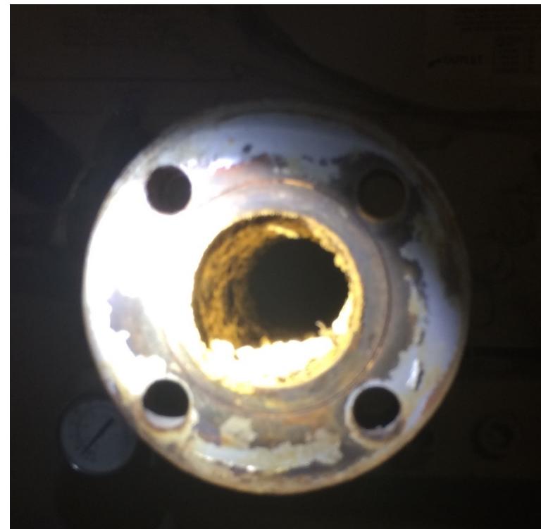
Inside Chilled Water Pipe with Corrosion
