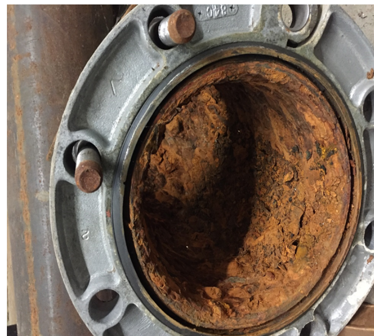
Interior Pipe Corrosion
