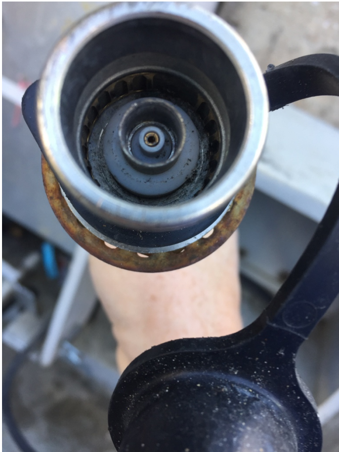
Same connector with corrosion in interior
