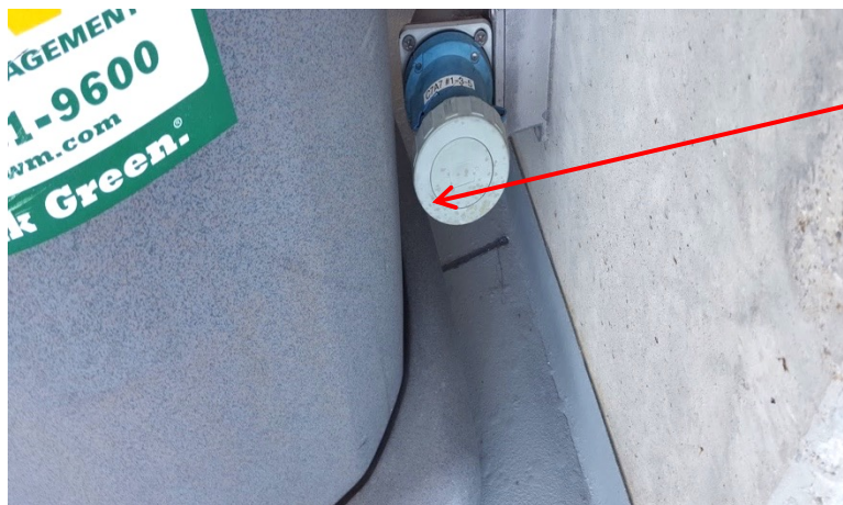
Damaged Portable Cart Connection
