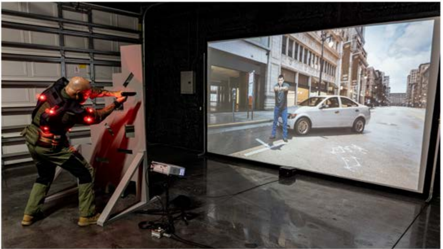
DART Red Fire works with third-party products like the SKIFTECH tactical vest and Scorpion shock band to simulate gun fire from characters within the simulation.
