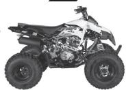
**ENGINE 125cc SOHC 4-Stroke** START METHOD Electric **COOLING Air cooled** TRANS. Automatic F-N-R **FUEL SYSTEM Carbureted** FRONT TIRES 19 x 7 x 8" REAR TIRES 18 x 9.5 x 8" **BRAKES Disc, front & rear** SEAT HEIGHT 271/2" WHEELBASE 391/2" DRY WEIGHT 227 lbs.
