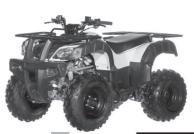
ENGINE 150cc SOHC 4-Stroke START METHOD Electric COOLING Air & remote oil cooler TRANS. 3 spd semi-auto w/reverse **FUEL SYSTEM Carbureted** FRONT TIRES 20 x 7 x 10" REAR TIRES 19 x 10 x 9" BRAKES Disc, front & rear SEAT HEIGHT 2834" WHEELBASE 411/4" DRY WEIGHT 310% lbs.
