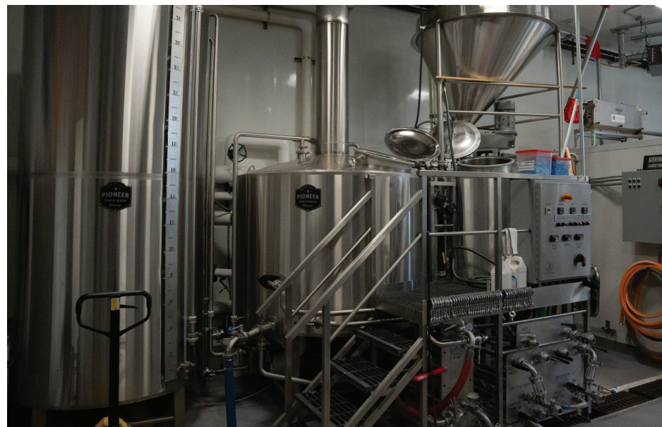
The three-vessel brewhouse at GILD, which consists of a hot liqueur tank, a brew kettle and a mash-lauter tun, on Feb. 5.
