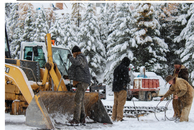
ABOVE: As snow continues to fall, mountain manager Pat McKay (far right) and a crew of maintenance workers at Snowbowl prepare to use a bulldozer to pull a Cat, used to groom the slopes, into position on a set of tracks. They are reassembling the machine on Nov. 4, 2022, after taking it apart during the off-season. MADDIE CRANDALL | MONTANA KAIMIN
