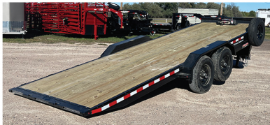
New H&H 22' Electric Tilt Winch, 14K GVW
