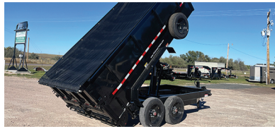
2026 H&H 14' Dump Trailer 48" sides, 8K axles, 18 Plys
