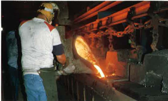
Molten metal is poured into the molds. About 100,000 parts can be made in a day.
