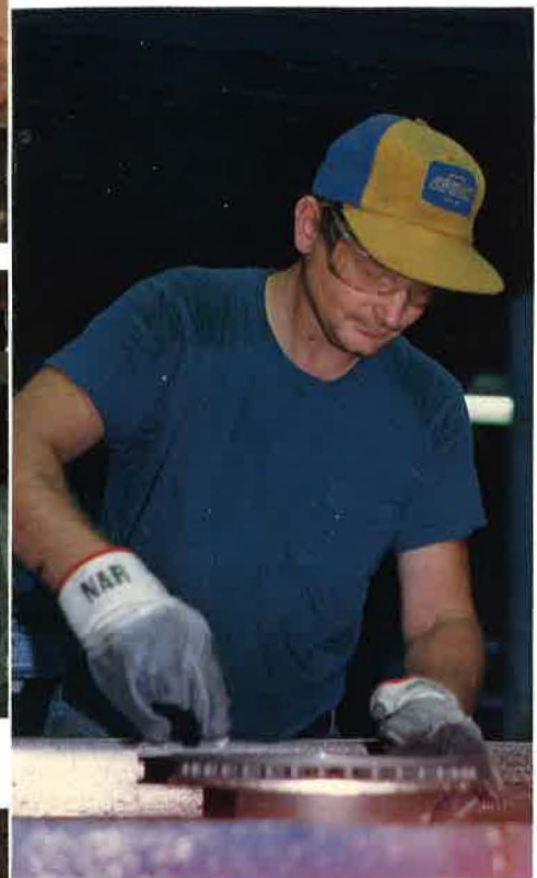
As castings cool, they are cleaned, processed, carefully inspected and shipped to customers.
