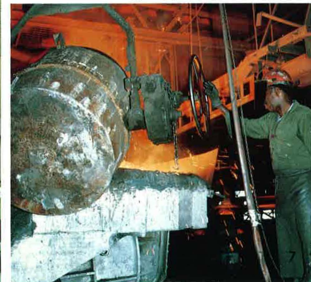
Quality is No. 1 priority. Metal is melted in a cupola, poured into an electric holding furnace, instantly analyzed by spectrograph.
