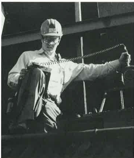
Preventive Maintenance Engineer Roger Hackett uses vibration analyzer to check wear and tear on a baghouse fan.
