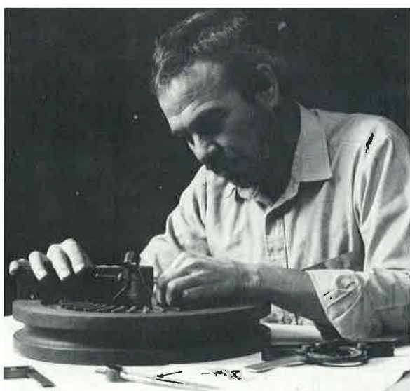
A craftsman at work. Pattern maker Joe Carter creates the intricate wood patterns used in making prototype castings.
