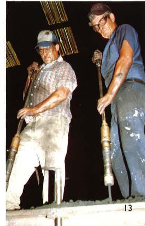
Wbeland's Jobbing Foundry makes some castings so large that the mold must be tamped by air hammers.
