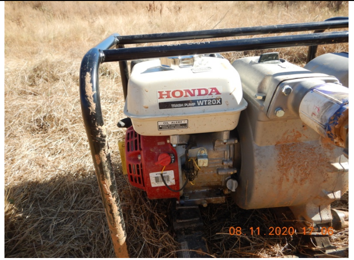
Photo 6. Honda WT20X trash pump which was used to pump sewage contained by bermed area back to lift station vault.
