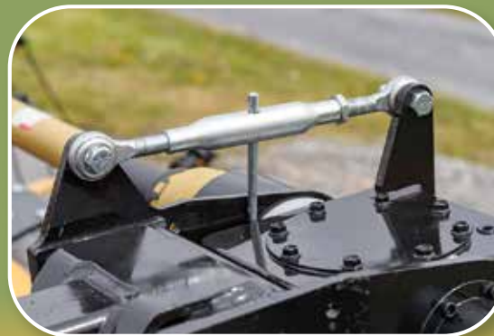
Tilt adjustment for light or heavy crop
