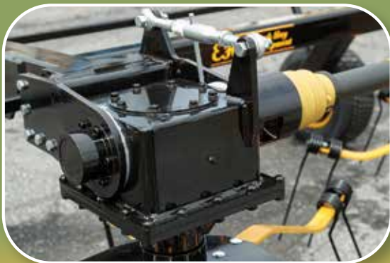
Individual oil bath gear box on each rotor.
