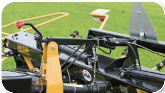
Hydraulic tilt allows operator to lift tedder over rocks, ridges, etc. while in operation
