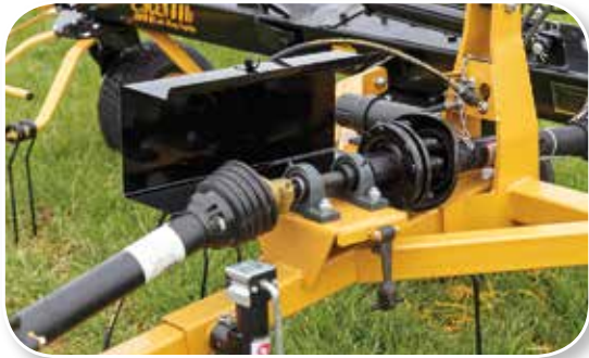
Heavy-duty double PTO shaft with friction clutch
