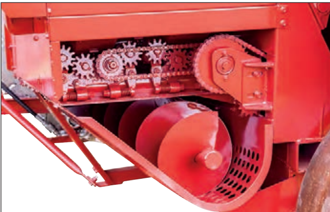
Large trash auger with perforated floor saves shelled corn from husking bed
