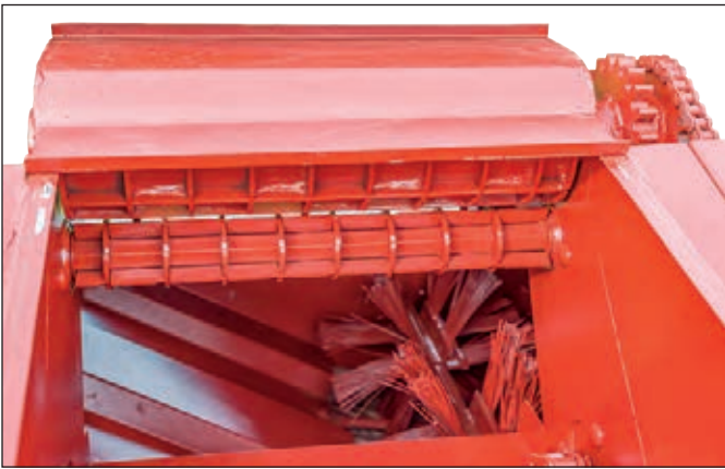
Aggressive trash rolls get rid of most trash before corn gets to husking bed
