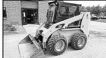
2012 Caterpillar 236B3: 2,565 hours, 1950 lb lift, cab w/ heat, pilot controls, 72" bucket, aux hyd, 4 cyl Cat C3.4 turbo, 7k lbs, stk#SK381, $26,500
