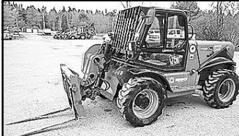
2013 JCB 520-50: 2,478 hours, 4400 lb lift, 16'5" lift height, 9'3" horizontal reach, 4x4, 42" forks, 4 cyl Perkins turbo, 77 hp, auxiliary hydraulics, stk#FL199, $34,500
