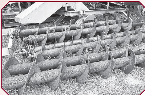
Industrial Augers (Flights Only) 12-1/2' and 30' (Total Lengths) 12-1/2' Flight- Flight Diameter 16", Shaft Diameter 6-3/4", Flight Thickness 3/8" 30' Long Flight- Flight Diameter 18", Shaft Diameter 6-1/2", Flight Thickness 3/8" Price: 12-1/2' $500 ea • 30' $1,000 ea
