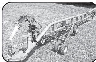
DRYHILL MULTIPURPOSE PUMPS 8" discharge, 540/1000 RPM
