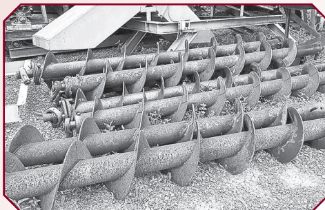
Industrial Augers (Flights Only) 12-1/2' and 30' (Total Lengths) 12-1/2' Flight- Flight Diameter 16", Shaft Diameter 6-3/4", Flight Thickness 3/8" 30' Long Flight- Flight Diameter 18", Shaft Diameter 6-1/2", Flight Thickness 3/8" Price: 12-1/2' $500 ea • 30' $1,000 ea
