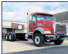
2013 Mack GU813 C&C Mack MP7 395 hp, Jake, Mack 10 Spd , 20/38k axles, Camelback Susp, 186" CT, 25' frame, 247k mi Stock# 5940
