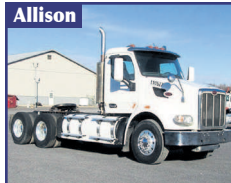
2016 Peterbilt 567 Cummins ISX12 (CNG ) 400hp, Allison 4500RDS, 15/46k axles, (Needs Repowered) 18k miles Stock# 5734
