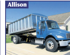
2017 Freightliner M2 SA Cummins ISB, 240HP, Allison, New Scott 16' Grain Dump, 12/21k Axles, 169k mi Stock# 5779
