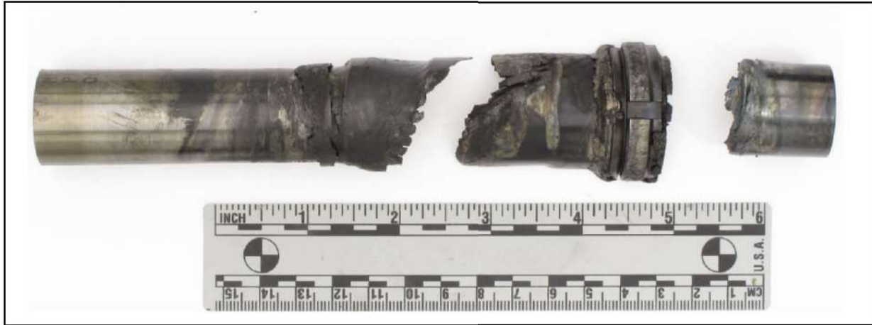
Figure 3. Turbine-to-compressor coupling shaft fractured. Photo courtesy Rolls-Royce.
