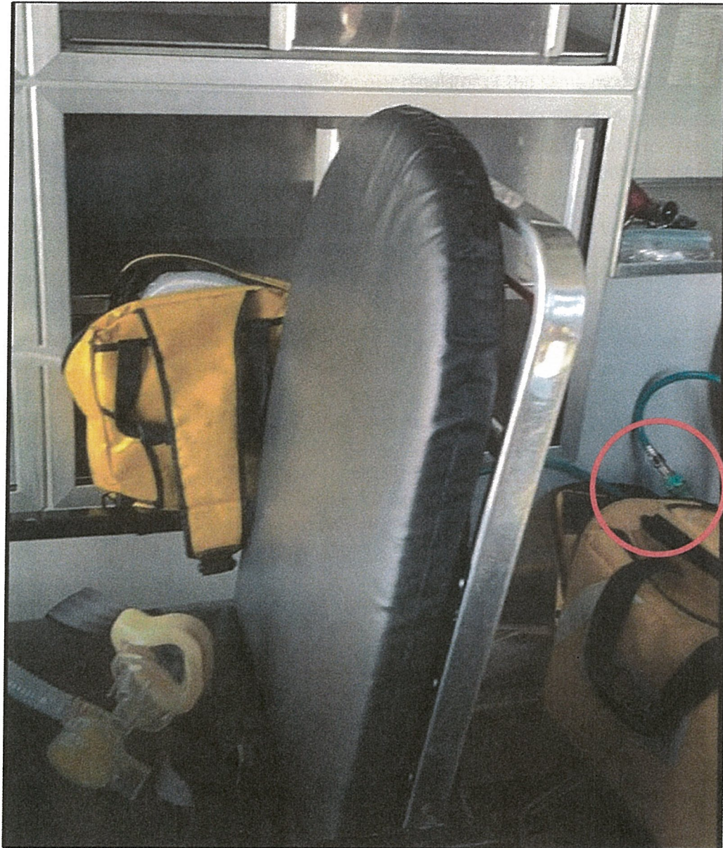
Figure 9) Possible position of the CPAP device and the position of the O 2 cylinder bag with the green O 2 hose connected to the pigtail linking the two pieces of equipment together (within the red circle) to enable O 2 flow to the patient via the CPAP device.
