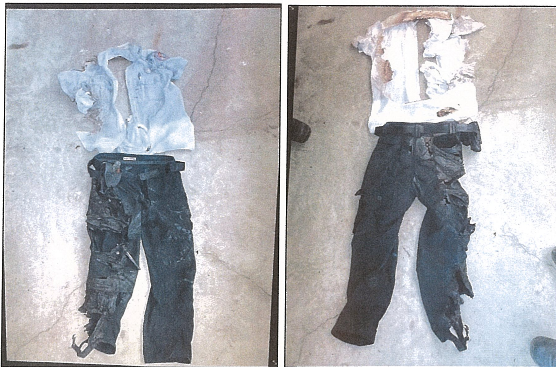
Figure 11A) The frontside of the paramedic's clothes worn during the fire with significant burns on the right side and noticeable less damage on the left side. 11B) The backside of the paramedic's clothes showing a distinct difference in damage between the right and left side as well as extensive thermal damage to the back of the shirt.
