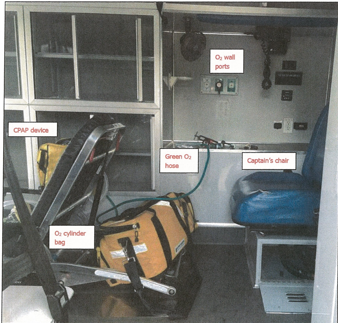
Figure 7) Photograph taken from exemplar ambulance's side door showcasing the most likely locations of the CPAP device, portable O 2 cylinder bag, the captain's chair, and the O 2 wall ports.
