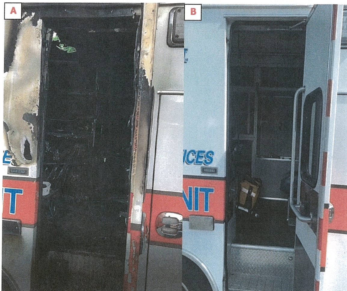
Figure 6A) Incident ambulance damage side perspective 6B) Exemplar ambulance from the same perspective.
