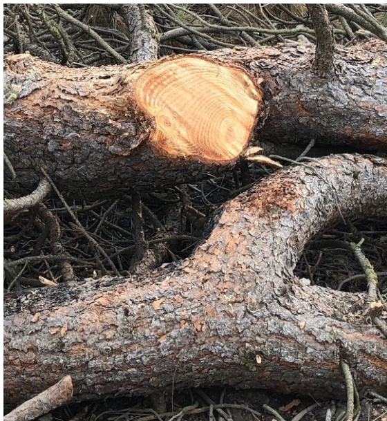
Figure 1. Cross section of the lateral branch/leader at juncture with stem revealing reaction wood.
