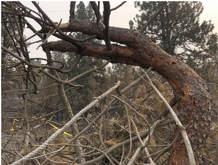
Figure 7. Portion of LBL, revealing split and cut ends, which failed prior to LBL implicated in Babb Road Fire.
