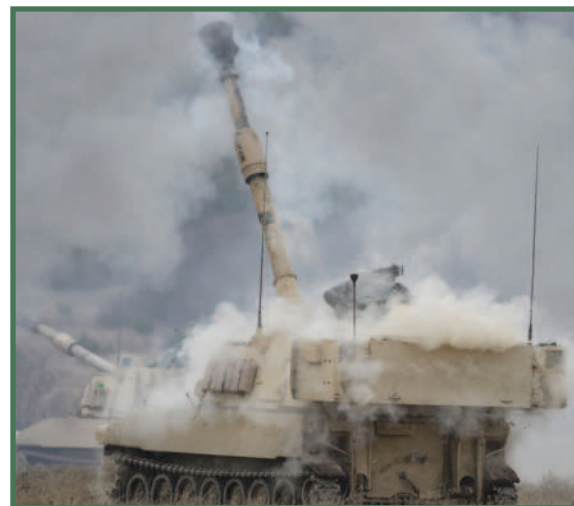
In 1942, artillery power came with a self-propelled 105mm Howitzer Motor Carriage M7. Today’s troops use the M109 Paladin, which carries a 155 mm Howitzer, seen below.
