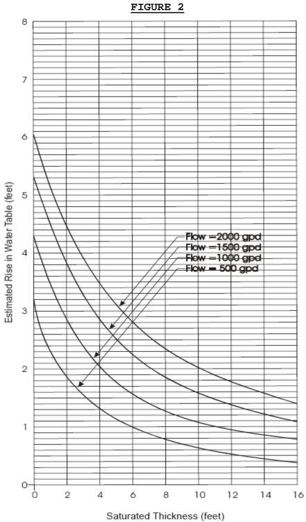
BASED ON A SOIL PERCOLATION RATE = 20 min/inch
