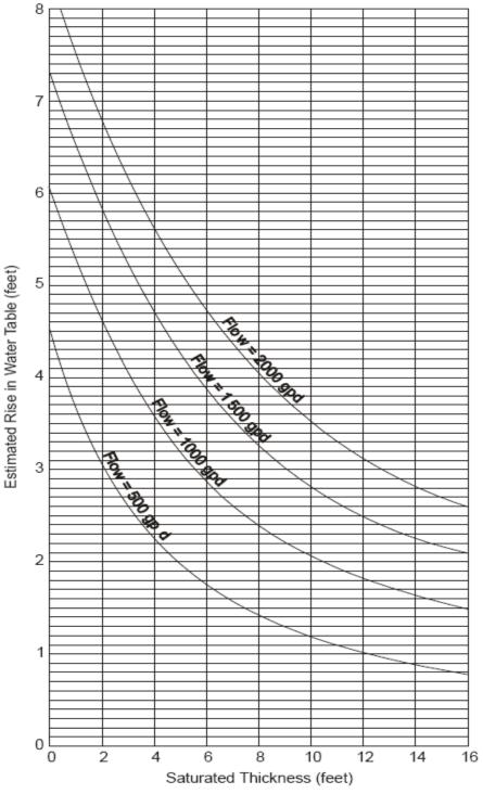
BASED ON A SOIL PERCOLATION RATE = 40 min/inch
