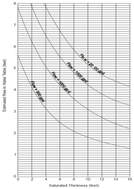
BASED ON A SOIL PERCOLATION RATE = 60 min/inch
