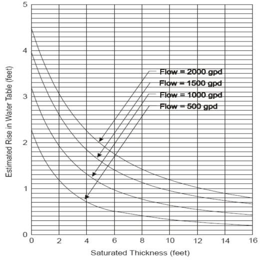
BASED ON A SOIL PERCOLATION RATE = 10 min/inch
