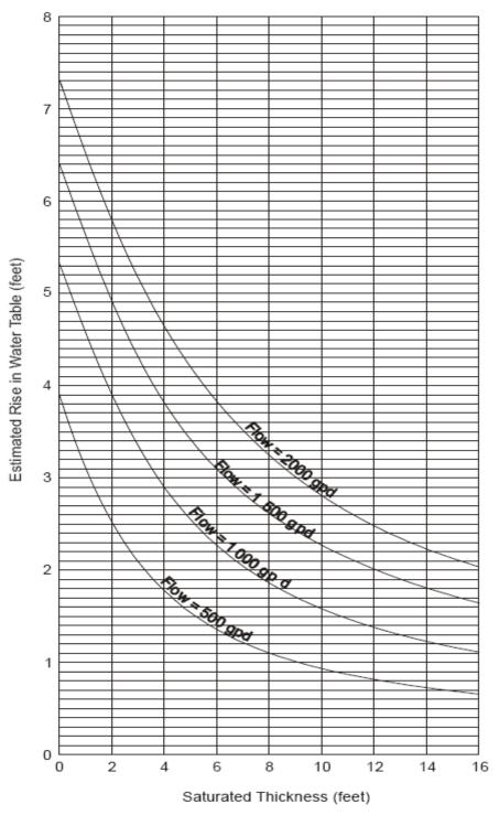
BASED ON A SOIL PERCOLATION RATE = 30 min/inch
