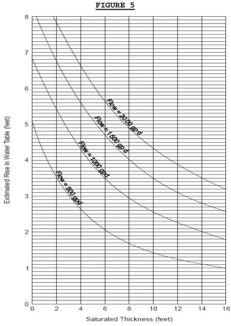
BASED ON A SOIL PERCOLATION RATE = 50 min/inch
