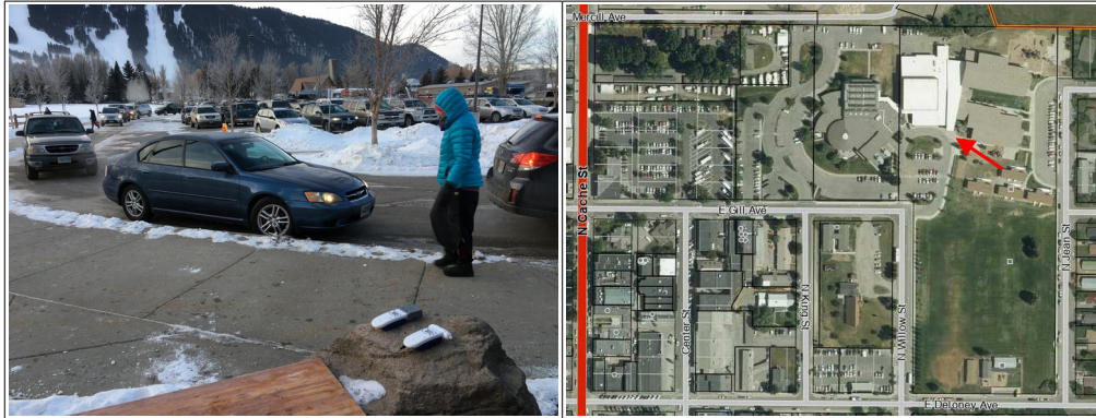
Figure 3.1: Air quality measurements were completed at the JES drop-off and bus staging areas on January 3 and 16, 2018. In addition to fixed positions such as shown (left), a technician walked with the monitors on the sidewalk near vehicles and buses.
