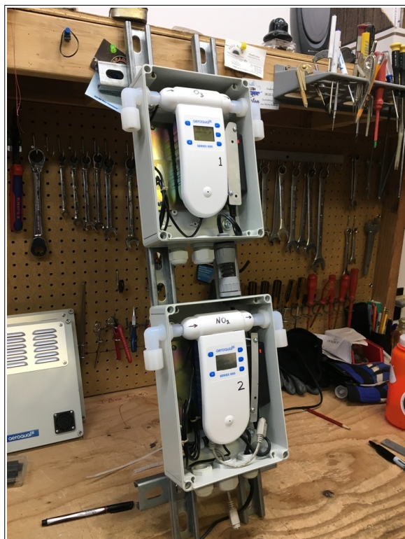
Figure 2.1: Aeroqual enclosures used for the Aeroqual S500 ozone and NO 2 monitors.
