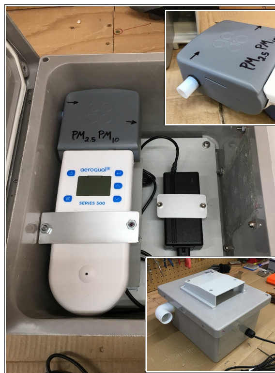
Figure 2.2: Custom enclosure used for the Aeroqual S500 PM 2.5 /PM 10 monitor.
