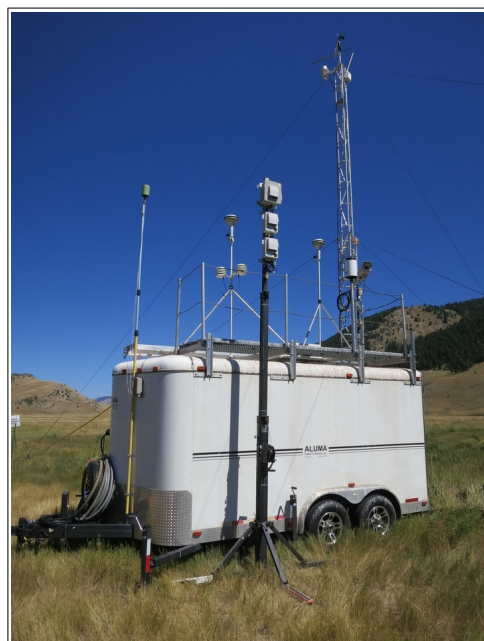
Figure 2.3: Aeroqual monitors (mounted on black crank-up tower) co-located with the WYDEQ Jackson Mobile in September, 2018.
