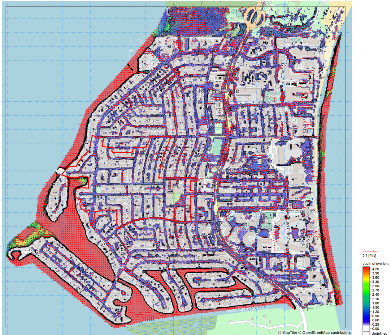
Figure 11 Model Simulation of Peak Flood Depth and Extent for 6/6/2022
