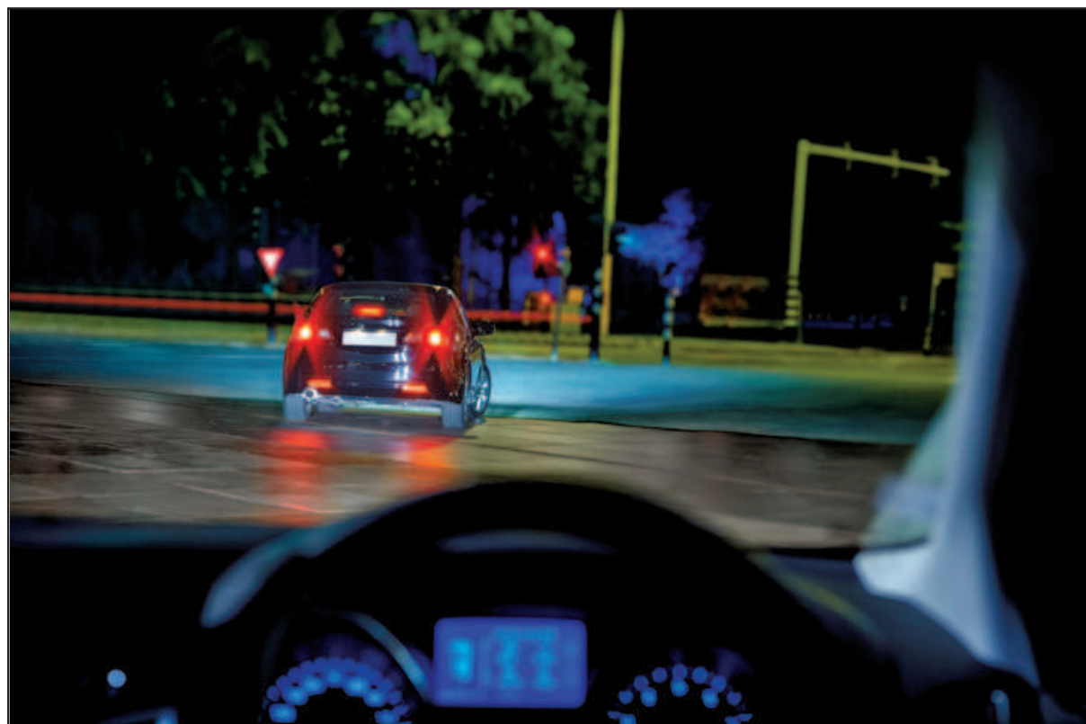
The instant-on response provided by Philips Vision LEDs can reduce braking distance by up to 20 feet at speeds of 75 miles per hour. Because they light up quicker, other drivers can see the vehicle sooner.
